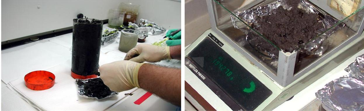
Figure 9. Removing and weighing sediment
