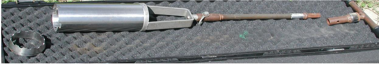
Figure 7. Sediment coring device
